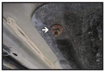
1. Using a 10MM deep socket, remove the nut from the underbody panel. Do this on both sides of the vehicle.
