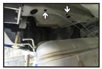
4. Feed lead wires from the small access holes in the frame to the large rear access hole as shown. Place spacer plates onto 1/2" x 1-1/2" carriage bolts. Attach lead wires to the end of the bolts. Do this on both sides of the vehicle.
